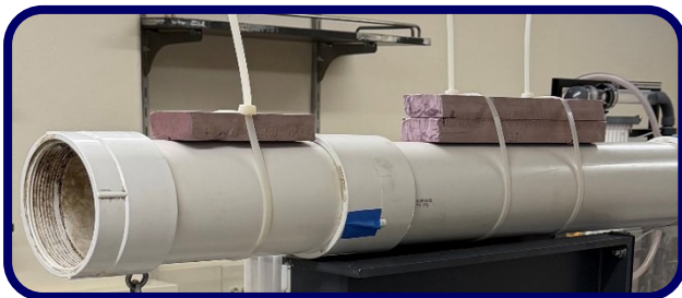
Project BALEEN milli particulate collector design for the testing phase at Spanish Lake Park, in which a conical filter is inserted into a long PVC pipe. A slab of dense foam is used to ensure neutral buoyancy – a useful feature for sampling below the surface.
